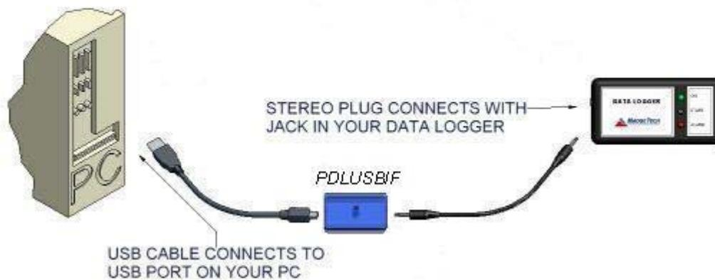
Insert the male connector of the PDLUSBIF interface cable into the female receptacle of the data logger. Insert the female USB connector into the USB.
