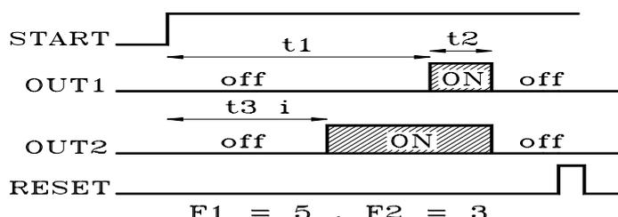
**F2 = 4 - Same function of OUT1 (time t1) with time t3 relative to t1 (in advance) :** The choice of this mode of operation enable the set "t3" that it has the same range time "S1" and cannot be higher of "t1."
